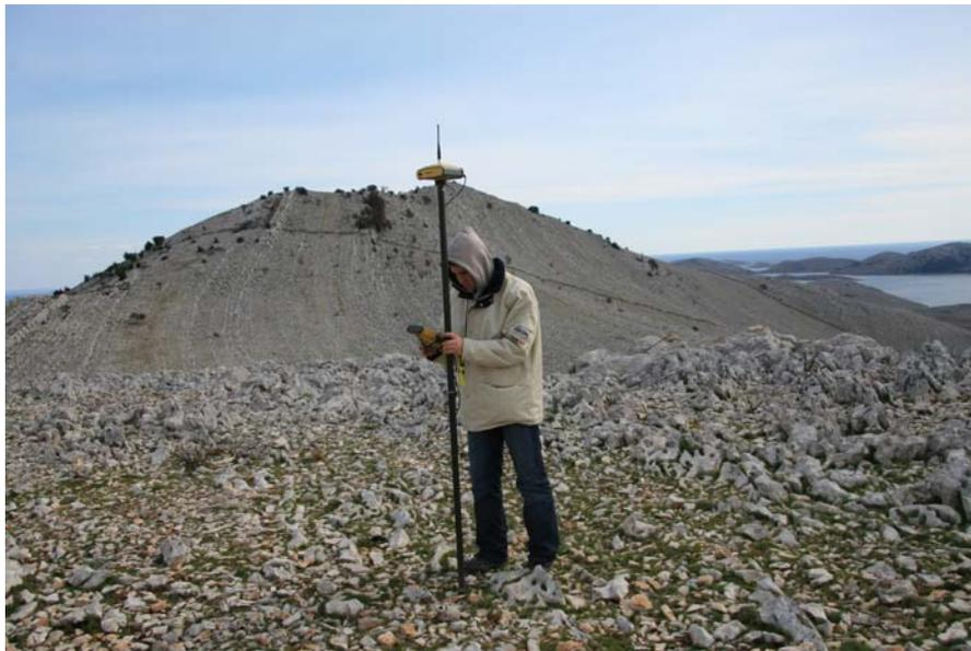
**FIG 3:** Data registrar Topcon FC-100 with Top SURV package
